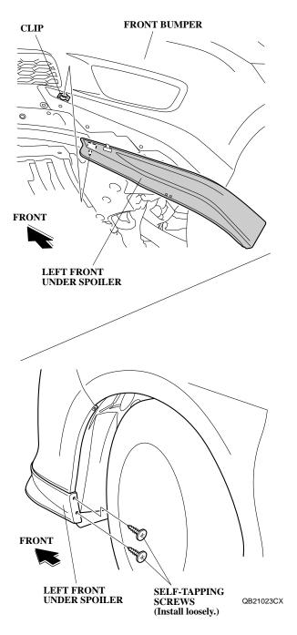
12. Check that the clip on the left front under spoiler is fully pushed into the slot on front bumper, then secure the front portion of the under spoiler to the front bumper with one washer and one bumper clip supplied.
