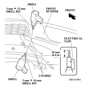
5. Install one clip into the upper 12 mm hole. Push in on the clip until you hear a click, then check to make sure the clip is secure in the front bumper.
