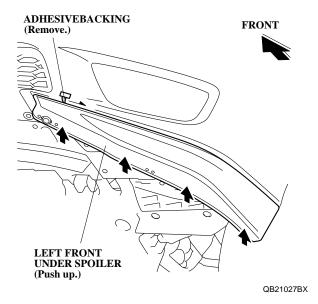
15. Using your hand, firmly press the left front under spoiler against the front bumper for 30 seconds.
