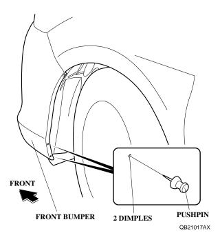
7. Thread a self-tapping screw into each pierced mark to make a hole in the front bumper. Remove the self-tapping screw.
